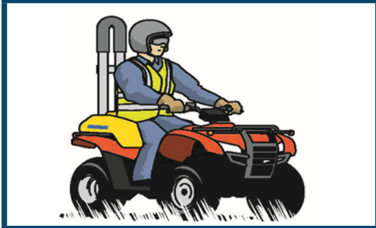
Figure 2 Quad bikes can be fitted with a crush protection device which may lower the risk of injury in the event of rollover.
